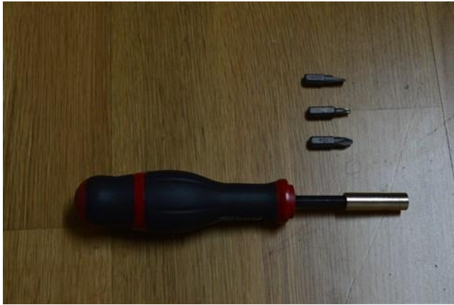
Torx 10, 20; flathead 10, socket wrench 13
