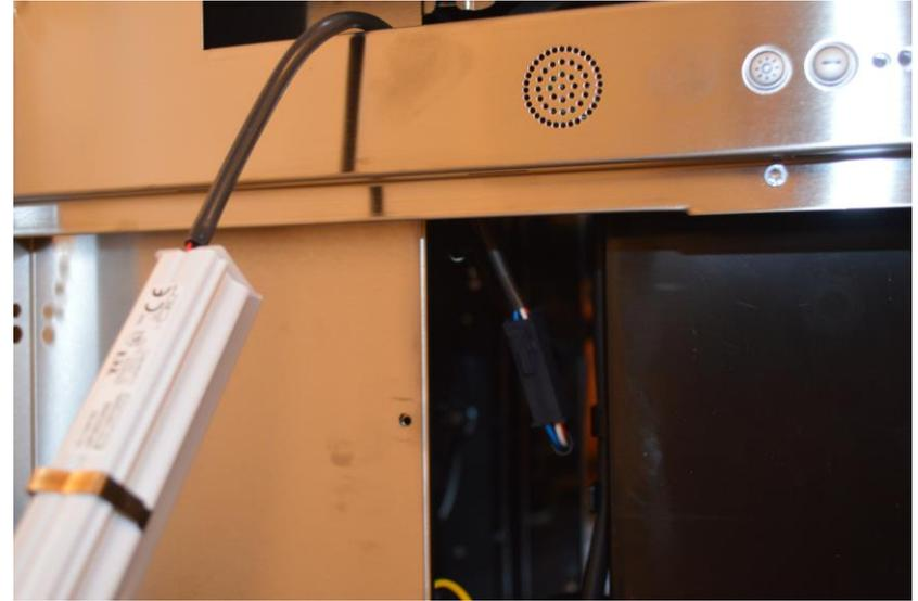
Remove the grease filter and lift-up the lamp with a flathead screwdriver and disconnect electrical connection remove the screws at left and right side / Togliere il filtro grassi, sollevare con un cacciavite piatto la lampada e disconnetter e la connessione elettrica
