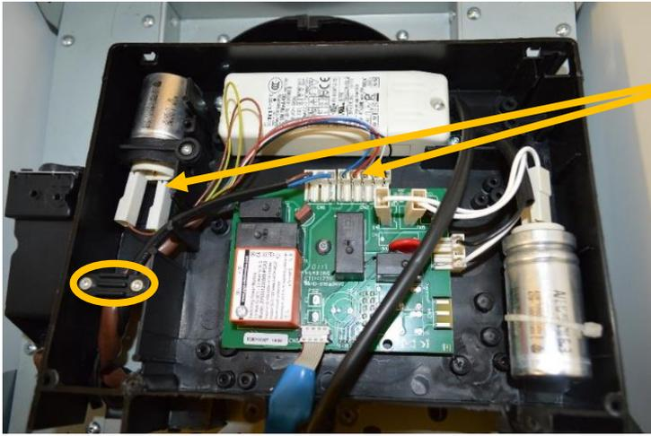
Open electronic device, remove cable fixing unscrewing n 2 screws. Disconnect Motor Connector from the main board and from capacitor. /
