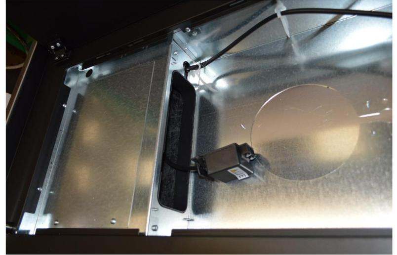
Remove the 4 fixing screws from the LED panel. Pay attention to illumination wiring, remove wire protection /
