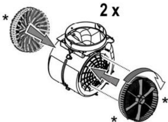
**Circular charcoal filter:** apply one on each side as cover to both the shield grids of the motor impeller, then turn clockwise. For the disassembly, turn counter-clockwise /
