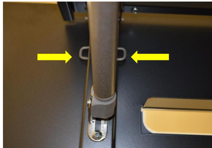
Unscrew n.2 screws for each piston to remove it. Remove the panel by pressing the springs. Attention: when replace front panel check the force in N , replace with the same force otherwise the panel could fall /
