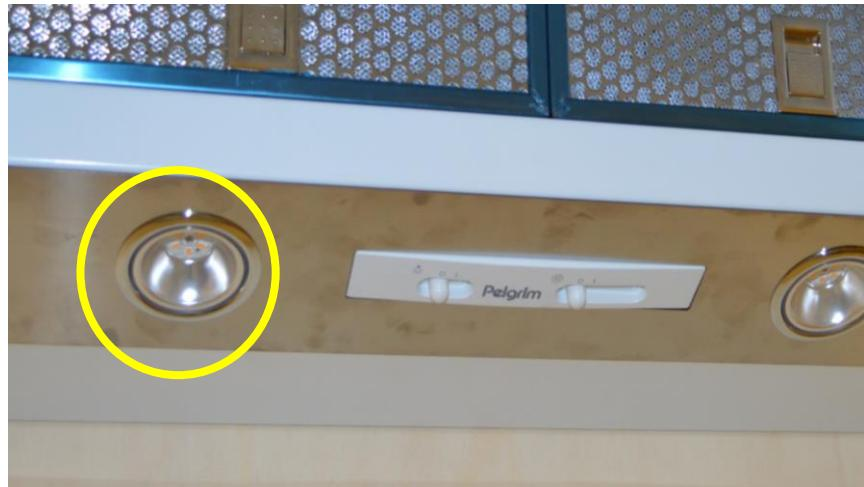
Remove the lamps by unscrewing them from their seat in case of halogen lamps; removing from the seat with a screwdriver in case of led lamps / rimuovere le lampade svitandole dalla sede in caso di lampade alogene. Rimuovere dalle sedi usando un giravite in caso di lampade led
