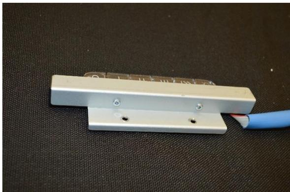
Unscrew the 2 fixing screws and replace user interface.
