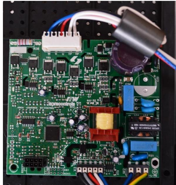
The board controls the brushless motor operation, receiving commands from the extraction board. There are 3 available connections: motor connection, power supply connection (L-N-ground) and communication connection. There are 2 LEDs directly positioned on the board: one red light and another green light. In the case of malfunctions, the Red LED flashes a certain number of times, in a way to communicate the type of problem:
