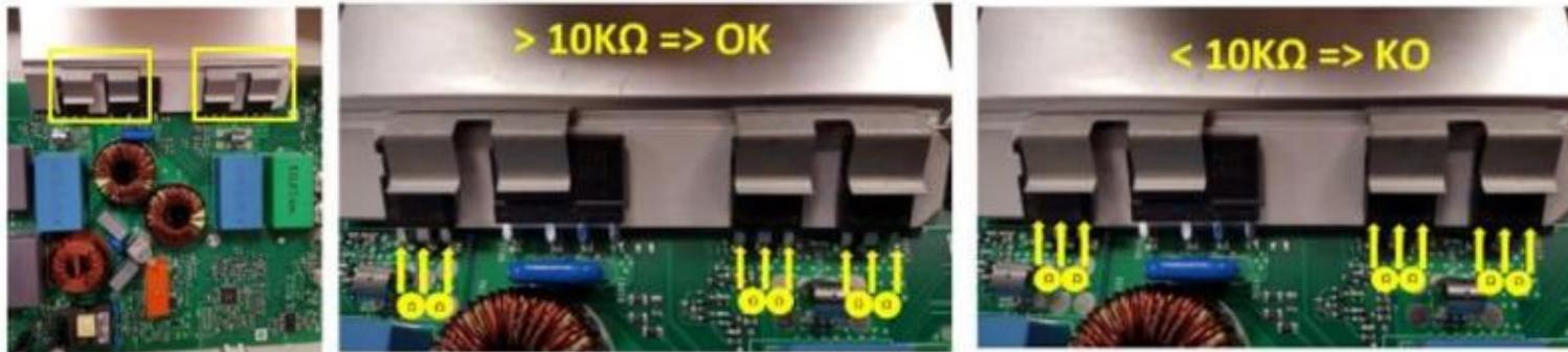
4. If the previous points are ok, disconnect the highlighted connector from the main board. If error D1 is displayed on the user interface of the extraction area (cooking zones are working properly but extraction is not, displaying error D1) replace the main board. If D1 is not displayed, repeat the operations indicated above, starting from point 1.
