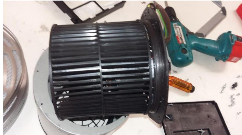
Unhook electronic wirings from the electronic device, Earth wirings and trasformer wiring to replace motor /
