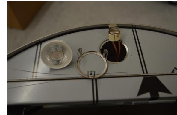
Lamp consists of 3 different parts: neon support; lamp; lampholder. Unhook the lamp from its seat and then remove also the lamp ring / La lampada è composta da 3 parti diverse: supporto neon; lampada; portalampada.
