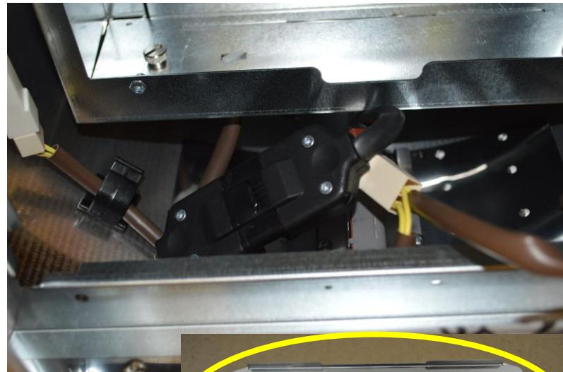
Tube Island has an openable service panel. Rotate 2 screws to access it
