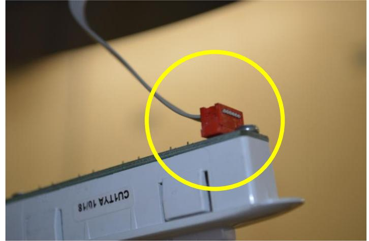
Pull out the cover and disconnect the connector / Estrarre la cover e scollegare il connettore
