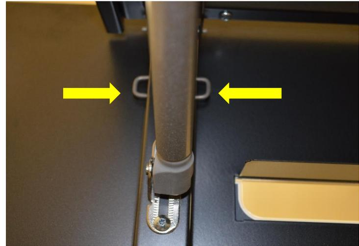
Unscrew n.2 screws for each piston to remove it. Remove the panel by pressing the springs. Attention: when replace front panel check the force in N , replace with the same force otherwise the panel could fall /
