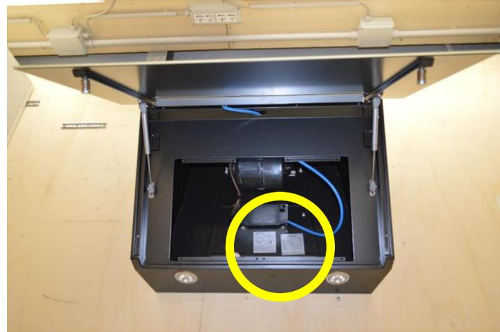
Remove grease filter and disconnect UI connector. Inside product it's possible to verify product labels and I2NC /
