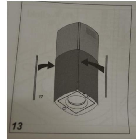
First install upper chimney and left outside mould, finally lower chimney and right outside mould /
