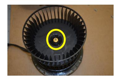
Unscrew 4 screws. Then remove the nut to set free the impeller.
