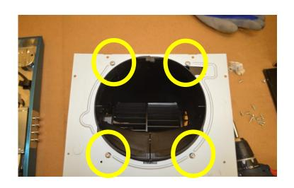
Lift up the superior motor panel. Then unscrew n.4 screws to divide motor from the panel
