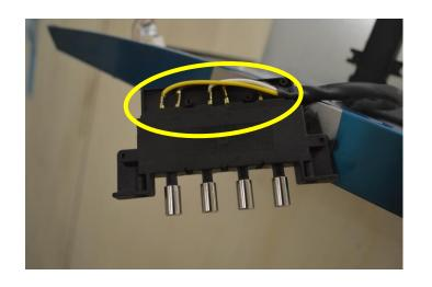
Remove 3 screws to open AGC box. Disconnect every fastons and replace UI
