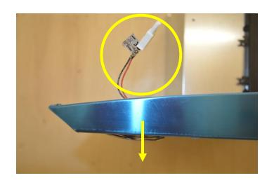
Disconnect lamp connectors. Press later metal spring then push down the lamp from it seat
