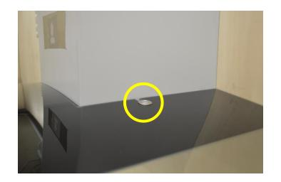
Remove 2 superior screws to remove glass panel and spacer
