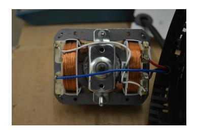
Unscrew 2 nut to remove the motor unit. Then detach all wires and weld them on new motor
