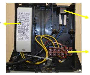
IEC Power Supply connector 230V
