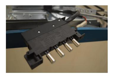
Remove 4 screws to unhook the AGC: 2 superior screws and 2 frontal screws. Then remove plastic cover
