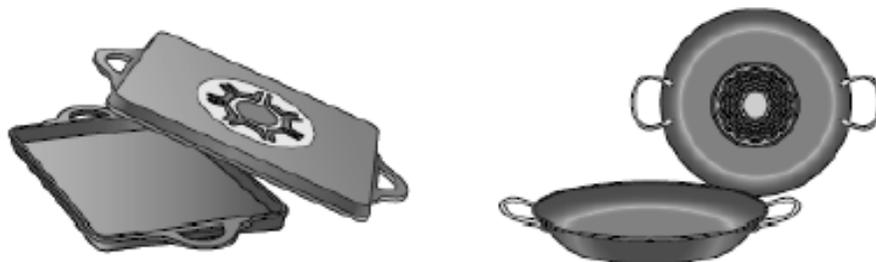
Pans with aluminium areas inserted in the base reduce the ferromagnetic area, so less heat may be supplied and the pan may be difficult to detect or not be detected at all.
